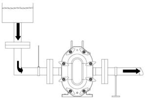
Figure 6: Correct Piping (Supply Above)
