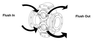
Figure 15: Proper Flushing for XP Double Seal
