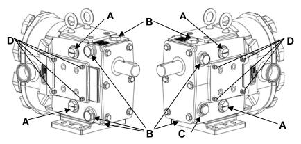
Figure 16: Lubrication Points
