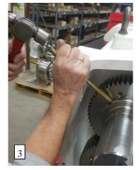
NOTE- Locknuts are installed with a minimum of 600 footpounds of torque using spanner type socket. A shaft locking device is used to stop shaft rotation when tightening.
