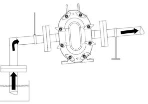
Figure 7: Correct Piping (Supply Below)
