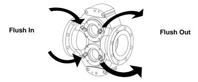
Figure 15: Proper Flushing for XP Double Seal
