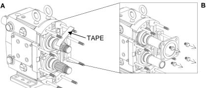
Figure 45: Tape Shafts and Remove Bearing Retainers
