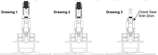
Figure 50: Pressing Rear Bearing onto Shaft
