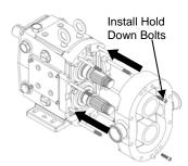
Figure 61: Installing Pump Body
