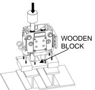
Figure 46: Pressing Shafts From Gear Case
