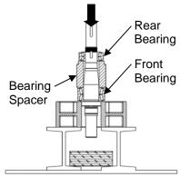
Figure 48: Removing Bearings and Sleeve From Shaft
