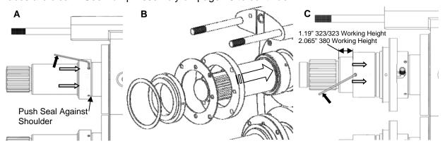
Figure 41: XP Double Mechanical Seal Assembly
