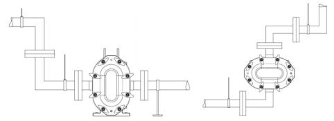
Figure 5: Piping Support Example
