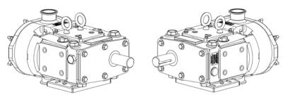
Figure 2: Shaft Mounts (Right and Left)
