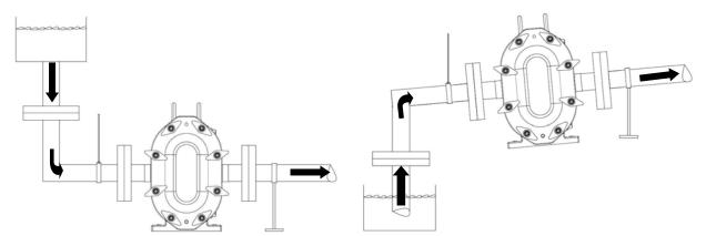
Figure 6: Correct Piping (Supply Above)
