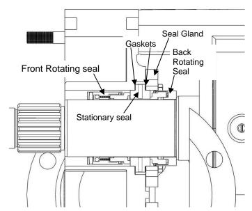
Figure 39: XP Double Mechanical Seal Disassembly
