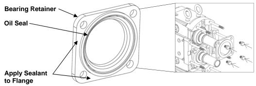
Figure 55: Bearing Retainer Installation
