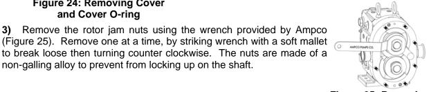
Figure 25: Removing **Rotor Jam Nuts**
