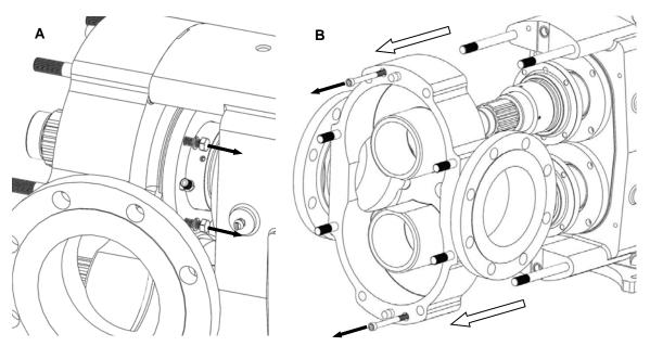
Figure 28: XP 320 Pump Disassembly
