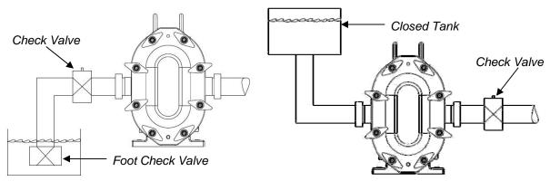
Figure 8: Check Valve (Inlet Side)
