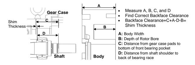
Figure 51: Calculating Shims
