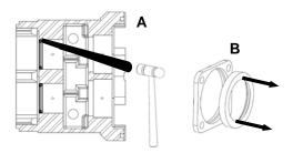
Figure 47: Removing Oil Seals
