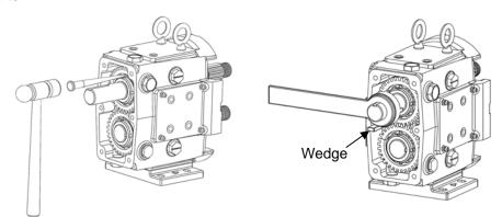
Figure 43: Bending Tabs on Lock Washers
