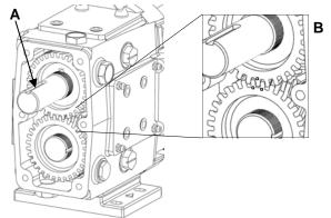
Figure 57: Installing Gears with Correct Timing
