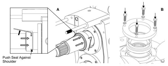
Figure 38: XP Single Mechanical Seal Assembly
