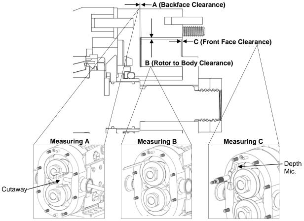
Figure 67: Critical Pump Clearances
