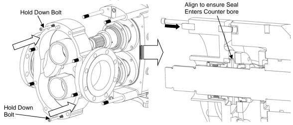
Figure 65: XP Installing Pump Body
