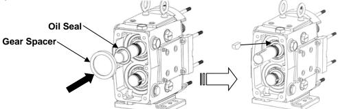
Figure 56: Rear Oil Seal and Gear Key Installation
