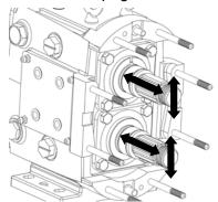
Figure 21: Check for Bearing movement
