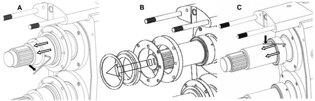
Figure 40: XP Double Mechanical Seal Disassembly
