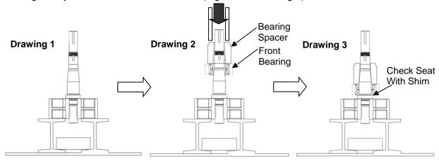
Figure 49: Pressing Front Bearing onto Shaft
