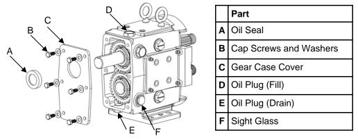
Figure 42: Gear Case Disassembly (Gear Case Cover)
