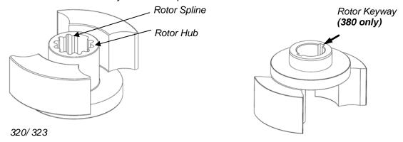
**Figure 19: Rotor Inspection Points**
