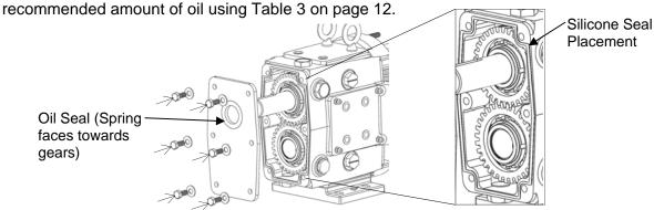
Figure 60: Installing Gear Casing Back Cover
