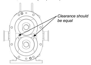
Figure 17: Clearance Between Rotor Tips
