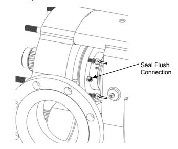
Figure 66: Installing Seal Gland and Flush
