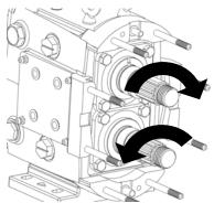
Figure 20: Check for Gear Backlash
