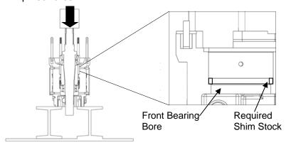
Figure 52: Pressing Shafts into Gear Case
