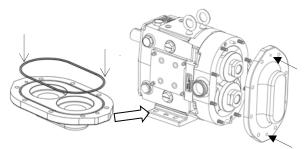
Figure 63: Installing Cover O-ring and Cover
