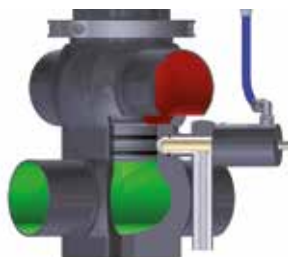
Two-way connection between main and CIP valve
