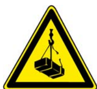
Warning: Suspended load.
