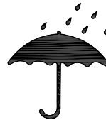
Against moisture protect
